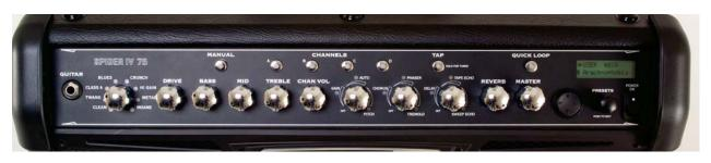
name of the alternate effect comes up on the LCD screen when you toggle the Preset knob. For example if you select the position labeled Phaser on the modulation effect knob, you can use the Preset knob to toggle to a Uni-Vibe effect. Choosing the labeled effect lights up a green LED, which switches to red as the alternate effect is chosen. Once you get the concept, it is pretty simple to choose your combination of three simultaneous effects (plus Reverb).
