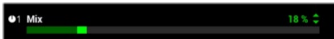
An automation assignment indicator for “Knob 1” appears at the left of the assigned slider
