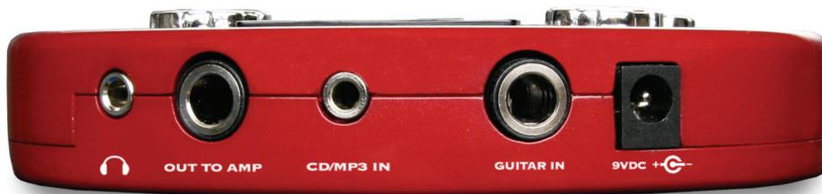
Your outputs include a 1/4-inch mono output to your guitar amplifier, and a 1/8-inch stereo headphone output for headphone jamming. Both outputs are controlled by the POD's Volume knob. Headphones are recommended for full stereo sound, but the Pocket POD Express sounds great feeding the input of a guitar amplifier as well.
